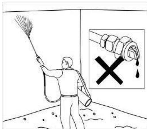
Clogged nozzles should be put in a container with water for several hours before the blockage is removed by a very soft toothbrush. NEVER clean nozzle with a hard pin or piece of wire and NEVER put a nozzle to your mouth to blow through it.
